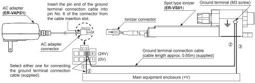
\* Pin No. 6 is connected to pin No. 5 (24V) of the ionizer connector.
