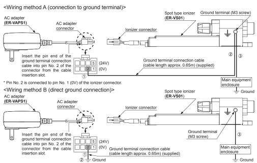
\* Pin No. 2 is connected to pin No. 1 (0V) of the ionizer connector.
